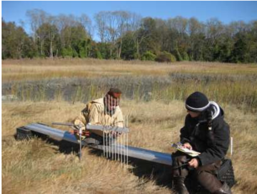
Figure 4: Photo shows the fourth pin being slid through the SET table to rest gently on the substrate surface for measurement. This is repeated four times at 90 degree angles for a total of 36 measurements and averaged to obtain a single SET data point (up to three times per year).
