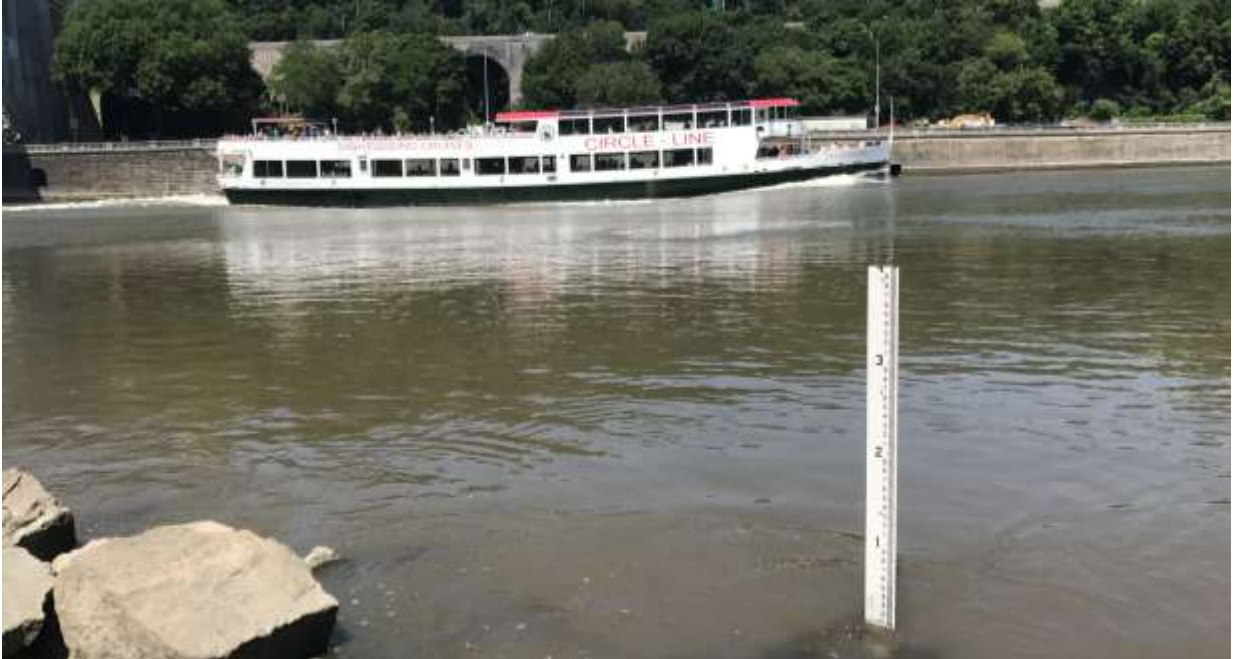
Figure 1. Example of a staff gauge (white scale attached to wood stake in the foreground) located in the water on the shoreline as a large boat passes Bridge Park on the Harlem River in the Bronx.
