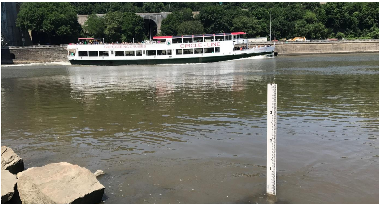
Figure 1. Example of a staff gauge (white scale attached to wood stake in the foreground) located in the water on the shoreline as a large boat passes Bridge Park on the Harlem River in the Bronx.
